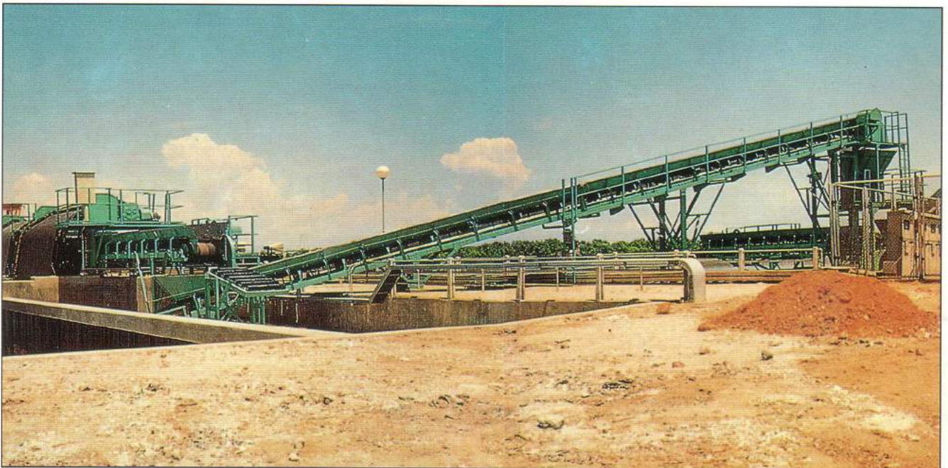
HORIZONTAL AND INCLINED BELT CONVEYORS
